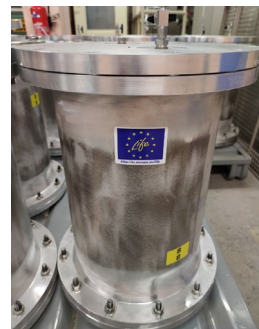
Cylindric vessels made with Aluminium specifically designed and used for the compatibility tests
