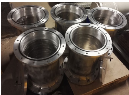
Cylindric vessels made with Aluminium specifically designed and used for the compatibility tests
